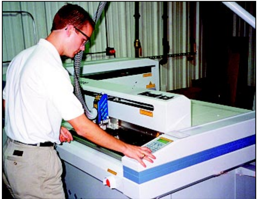
Chris Shiflett adjusts a sheet of acrylic on K&A Crylic's new laser in preparation for it to cut and finish a product.
